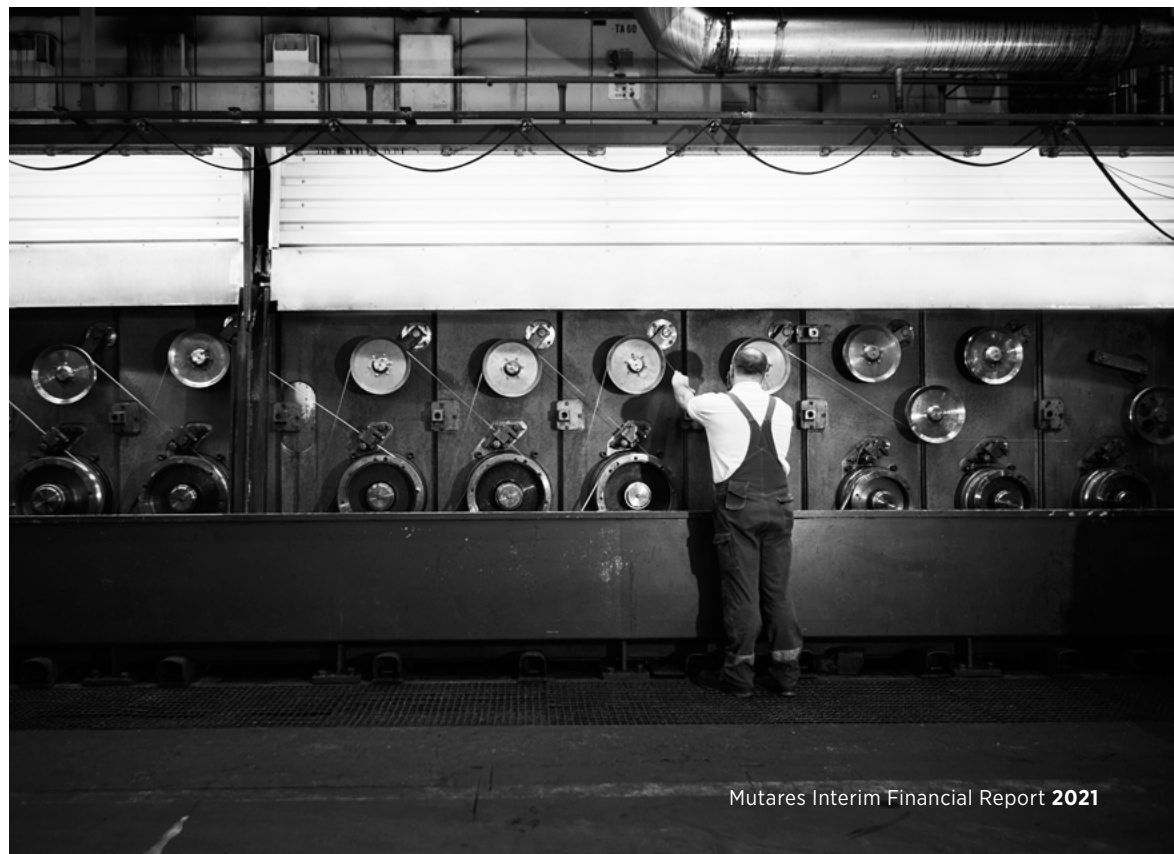
Employee checking machine, which is making copper wire thinner by extending it
