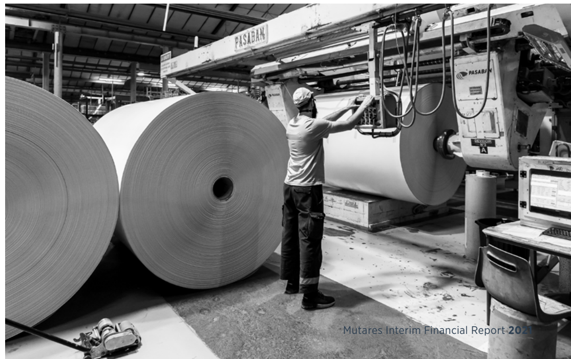
Cutting machine bringing the cardboard in the right format
